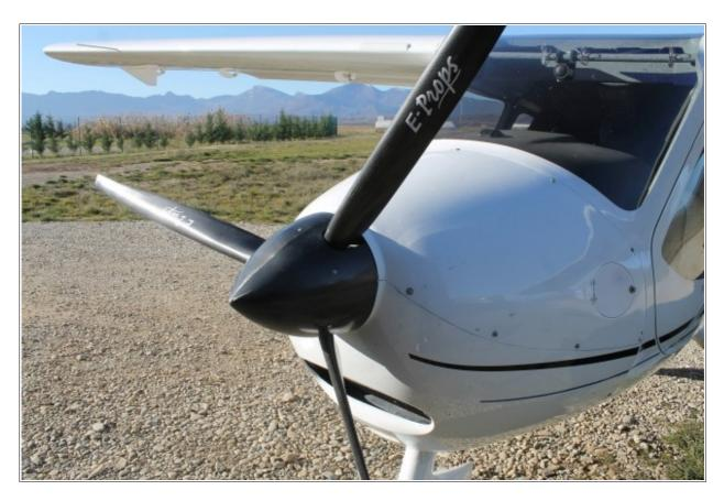
A detailed comparative has been realized on the CTLS equipped with a Rotax 912S engine (100 hp) between the standard composite 3-blades NEUFORM diameter 165 cm and the E-Props 3-blades propeller DURANDAL 100-M (diameters 170 or 175 cm depending on CTLS versions).
